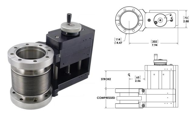
The newest member of the Hositrad CF translator family, the HO\_BLT45S has the cantilever brackets (see drawing above) bolted to the side of the flange. The advantage here is that the cantilever brackets leave 75% of the circumference of the flange unobstructed. This allows the translator to mount in very close quarters without interfering with other, nearby flanges.
